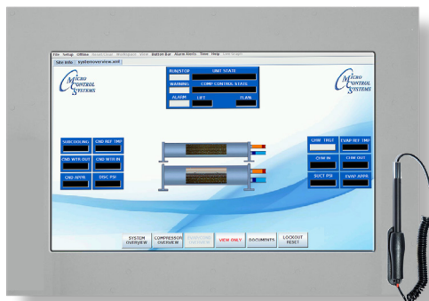
EVAPORATOR CONDENSER OVERVIEW SCREEN
